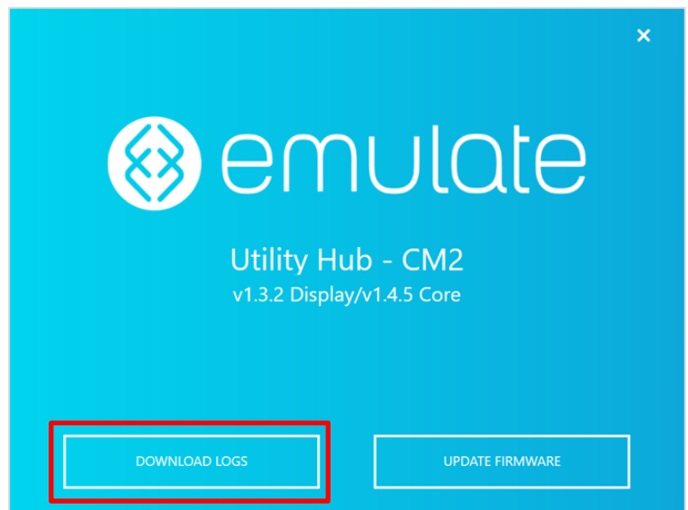
Figure 26 | The Utility Hub home splash screen for Zoë-CM2 showing the option to Download Logs and Update Firmware . The Utility Hub home splash screen for Zoë-CM1 looks nearly identical, the only difference is the version numbers displayed in the center of the screen.
