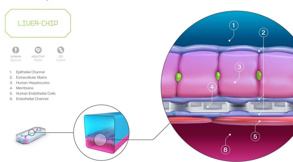
Liver-Chip Culture. Primary human hepatocytes were cultured in the upper channel and on the top of the ECM-coated membrane, and primary liver sinusoidal cells (LSECs) were cultured in the lower channel and on the opposite side of the membrane. Cells were allowed to acclimate for approximately 1 week prior to compound treatment using flow rates of 10 to 30 uL/hour
