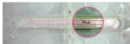
Small bubbles in Top Channel
