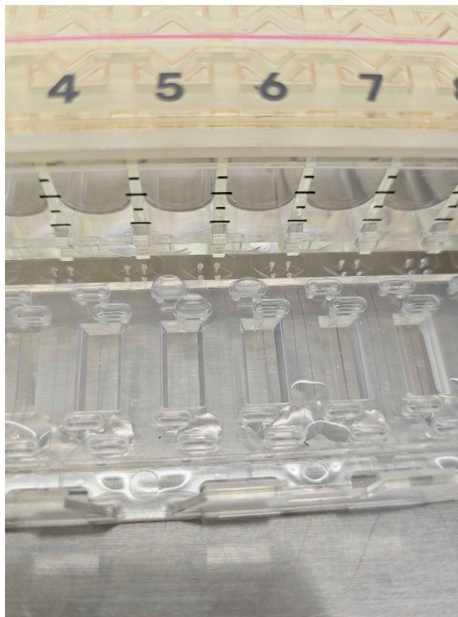
Figure 19. Successful priming indicated by media visible in the gasket port cavities.
